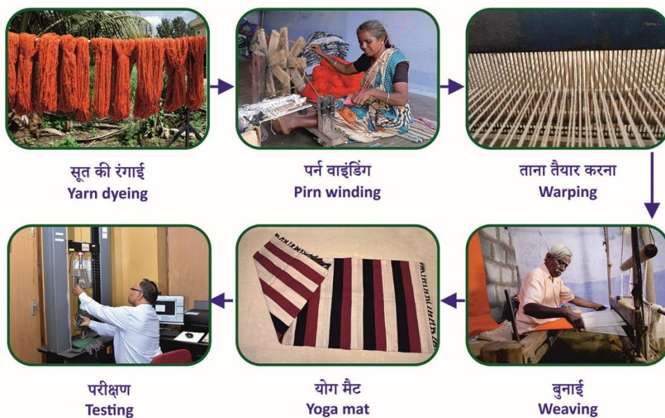
Fig.5. Weaving and testing the yoga mats
