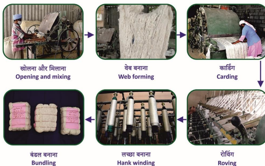
Fig.3. Spinning process of recycled silk yarn
